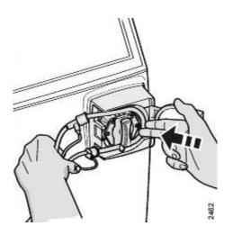
Place the blood pump segment over the blood pump rotor as shown in the corresponding figure.
