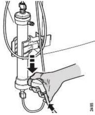
2. Keep the button on the dialysis fluid tube pressed and hold while attaching it to the dialyzer connector as shown in the corresponding figure.
