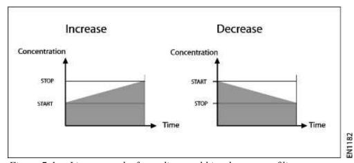
Figure 7:1 Linear graphs for sodium and bicarbonate profiling
