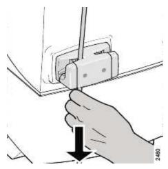
Then pull the blood line lightly downwards; the line goes into place when it is lightly pressed at the same time.
