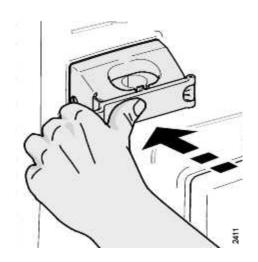
The air detector cover may be opened with ease by pressing the middle of the cover at the same time as the cover is being opened, as shown in the corresponding figure.
