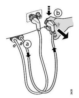
**To remove** the dialysis fluid tube from the safety coupling; **press and hold the button on the dialysis fluid tube** as shown in the corresponding figure ( ), before removing it from the safety coupling.
