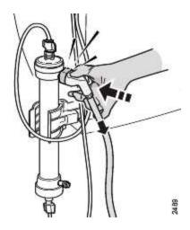
6. Release the button and simultaneously push the connector into place until it clicks in. Make sure that it clicks in properly to prevent leakage during treatment.
