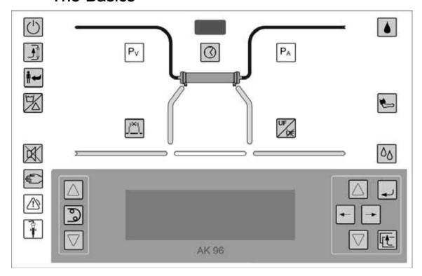
The Operator's Panel of the AK 96 dialysis machine consists of; a time display at the top of the panel, a Flow Diagram below this, function buttons, a key pad (setting keys) and an Information Display. The purpose of these components is to inform the operator of status and parameter values and also to guide the operator through the various procedures.
