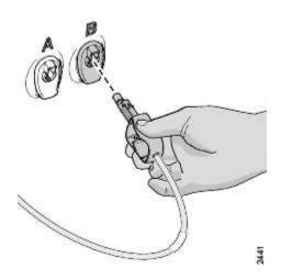
7. **Blue Concentrate Connector with White Tube Marking** This connector is used for the separately attached pick-up tube for liquid bicarbonate or acetate concentrate.
