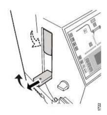
19.b. Close the upper latch by folding it in. Close the lower latch; pull out the latch and fold it in.
