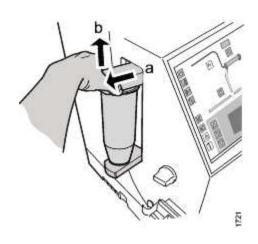
19.a. Open the upper latch of the BiCart holder; pull out the latch ⓐ and lift upwards to its uppermost position ⓑ . Remove the BiCart cartridge.
