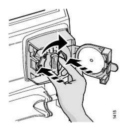
To attach the blood pump rotor; whilst holding the handle, place the rotor on the pump shaft. Then move your fingers from the handle and place them on the rotor as shown in the figure. Turn the rotor clockwise slowly, and at the same time push slightly, until it reaches the bottom position. Continue turning until the blood pump handle clicks in.
