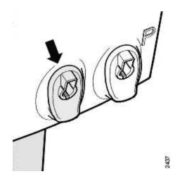
5. **Disinfection Port for Yellow Disinfectant Connector**The yellow disinfectant connector (point 6 in this list) is to be connected to this yellow port when a chemical disinfection program is performed. This is on condition that the disinfectant used for chemical disinfection program is permanently connected to the inlet line at the back of the machine (see "The Rear of the Machine" on page 2:28 in the next section).
