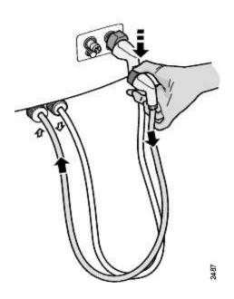
4. Disconnect the inlet dialysis fluid tube from the safety coupling of the machine; remove it in the same way as the outlet dialysis fluid tube described in the former point 1 in these instructions. The spent dialysis fluid flows to the machine from the dialyzer via this tube. A small arrow, fixed just below where the tube comes out from the machine, shows the flow direction.
