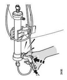
3. Release the button and simultaneously push the connector into place until it clicks in. Make sure that it clicks in properly to prevent leakage during treatment.
