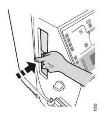
19.c. Check that both the latches of the BiCart holder have been properly closed.
