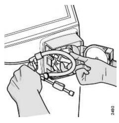
21.2. Open the cover of the air detector (press on the middle of the cover at the same time as the cover is being opened). Compress the venous drip chamber and then pull it out as shown in the corresponding figures.
