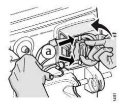
Continue turning the blood pump rotor in an anti-clockwise direction, while holding the segment, to thread the segment through the blood pump. The pins on the blood pump rotor, pointed out as a in the figure, hold the segment in place.
