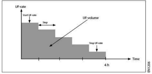
Figure 7:3 Decreasing graph in steps for UF rate profiling
