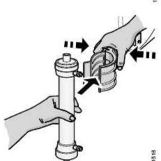
If necessary, squeeze the spring-clip as shown in the corresponding figure, to place the dialyzer in the holder.
