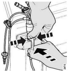
Compress the venous drip chamber as shown in corresponding figure and push it in to the air detector.
