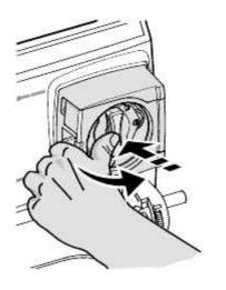
The pump cover may be opened with ease by pressing the middle of the cover at the same time as the cover is being opened, as shown in the corresponding figure.
