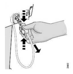
To remove the connector from the port; compress the connector as shown in the corresponding figure, before pulling the connector out.
