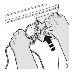
Close the blood pump cover by pressing at the point shown in the corresponding figure.
