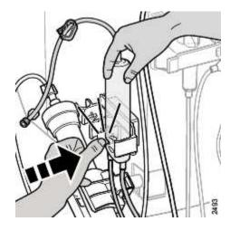
1. Place the venous expansion chamber in the holder in an upright position (inlet and outlet facing downwards). Make sure that it clicks in properly in the expansion holder.
