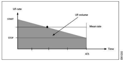
Figure 7:2 Decreasing linear graph for UF rate profiling
