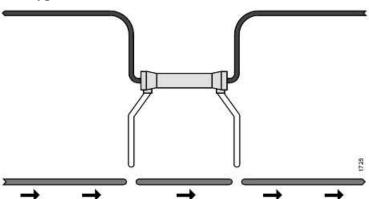
The bypass path lights green when the dialysis fluid preparation is ready (the conductivity level of the dialysis fluid is correct) for treatment. When the dialysis fluid is not correct the path is orange. The machine will automatically bypass the dialyzer during certain alarm conditions and during self-calibration.
