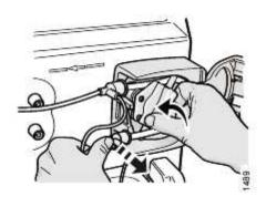
21.1. Clasp on the arterial blood line just before the pump segment. Pull it out while simultaneously turning the blood pump rotor in an anticlockwise direction. Make sure that the pins on the blood pump rotor are behind the pulled out segment while turning the rotor.
