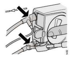
Make sure the blood pump segment collars are outside the pump housing.
