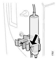
2. The edge inside the holder should fit into the groove of the expansion chamber as shown in the corresponding figure.
