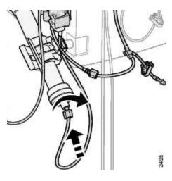
4. Connect the blood line with the expansion chamber to the dialyzer.
