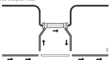
The dialyzer path lights green when dialysis fluid is passing through the dialyzer.
