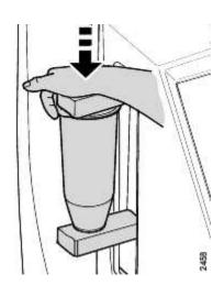
2.c. Bring down the upper latch and place the top port of the cartridge into the hole of the upper latch. Press down the upper latch to puncture the cartridge.
