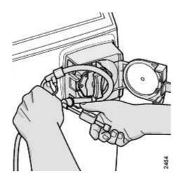
Place and hold the blood pump segment in the way shown in the corresponding figure.
