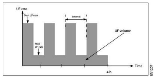
Figure 7:4 Graph in intervals for UF rate profiling
