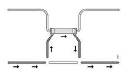
The dialysis fluid will now enter the dialyzer when the dialyzer path on the Flow Diagram lights up green. Especially note that the dialyzer should be filled from bottom to top to ensure proper de-airation.
