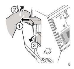
2.b. Place the bottom port of the BiCart cartridge into the hole of the lower latch as shown in the corresponding figure.
