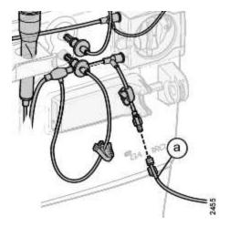
There is also the possibility of connecting the infusion line to the extracorporeal blood circuit pre-blood pump, i.e. before the blood pump. The corresponding figure shows pre-blood pump connection of infusion. The infusion line is marked ⓐ.
