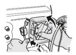
Press on the blood pump segment at the point shown in the figure before turning the blood pump rotor in an anti-clockwise direction. This is to hold the segment collar outside the pump housing while threading it.
