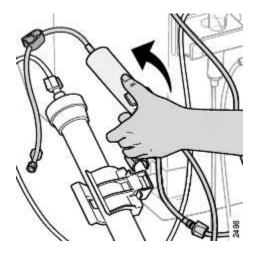
5.a. Tilt the expansion chamber holder backwards until it clicks into position. By doing so the venous expansion chamber will be filled to a suitable level during priming.
